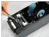
Reflective sensor (Black Mark Sensor)
