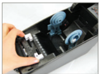
Transmissive sensor (Gap, Media sensor)
